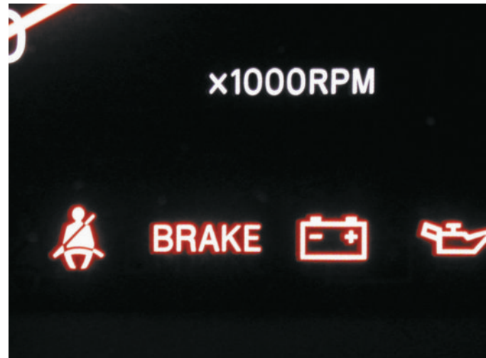
FIGURE 92-5 The red brake warning light will remain on after a bulb test if there is a fault with the hydraulic part of the brake system.
